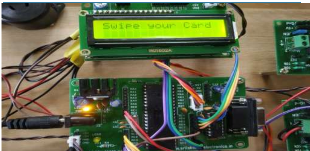
b) RFID Tag using EM 18, it wills going to scan the card
